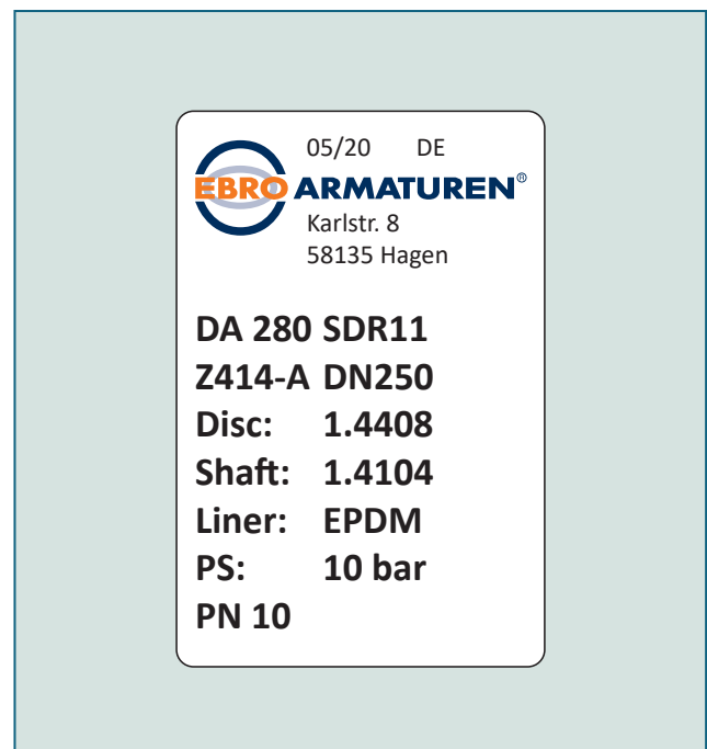
Type plate for clear identification of the Z 414-A.
